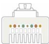
Figure 1-4. CAT5/5E/6 Straight Through UTP/STP Cable (8P8C)
